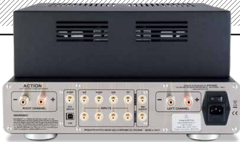
ABOVE: Four line inputs on RCAs are joined by coaxial and USB-B connections for digital sources. Rather than offer separate 4ohm/8ohm taps, the Action A100 Titan is equipped with single (6ohm rated) 4mm speaker outlets [see Lab Report, right]
